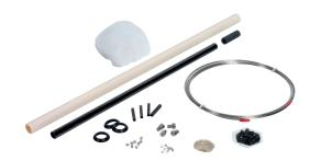
Both kits contain the same amount of consumables for 3,000 analyses in a TC/EA and Flash 2000 HT or Flash HT *Plus*, respectively. 'The only difference between the two kits is the length of the ceramic tube of the reactor: 450 mm for TC/EA and 470 mm for Flash HT and Flash HT *Plus*.
