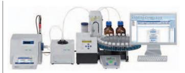
Density, refractive index (or related values), pH (or conductivity), acidity and color can be measured and analyzed in one go.
