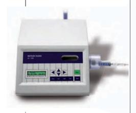
The DA-100M density meter is a compact three-decimal place density meter. It is equipped with a solid state thermostat and an air pump to dry the measuring cell. The optional ASU-100 sampling pump greatly simplifies density determinations of low viscous samples.
