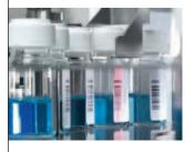
LiquiPhysics Excellence is not only able to read barcodes; it can also accurately interpret their information. With Smart Codes containing information about the type of product to be measured, the operator simply scans in the barcodes to start the measurements. No additional button to click.
