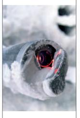
FBRM® C35 monitors real-time changes in particle count and dimension during cohesive wet or dry particle processing. In situ measurements enable Quality by Design (QbD) throughout granulation development, scale-up and manufacturing while ensuring the targeted granule size is achieved.
